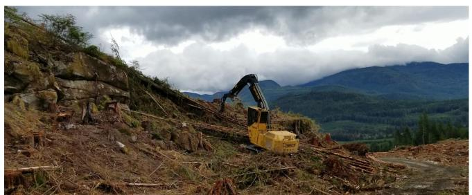
Above: A log loader hoe chucking logs to roadside. Courtesy of Steve Henderson.
