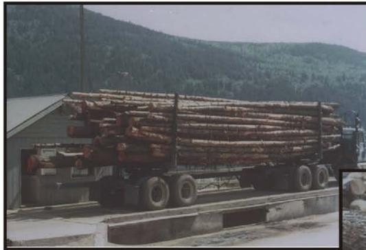
*A loaded truck on a weight scale.*
