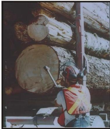
*Hammer indenting a log with a timber mark.*
