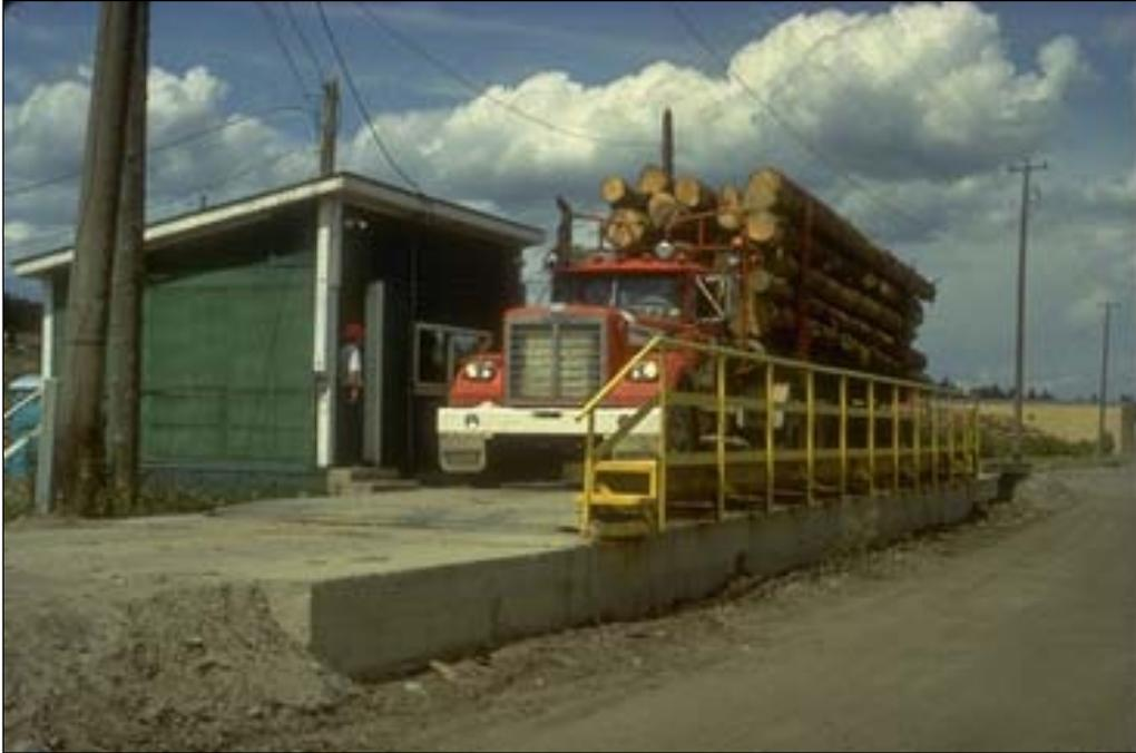
*Figure 13.1 A Loaded Logging Truck on the Platform of a Weight Scale.*
