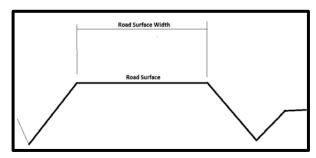
Figure 2 Road Prism Diagram
