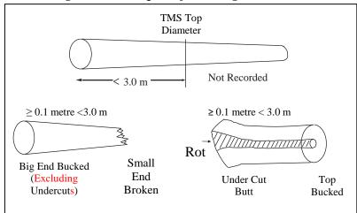
Figure 10 Examples of Bucking Waste
