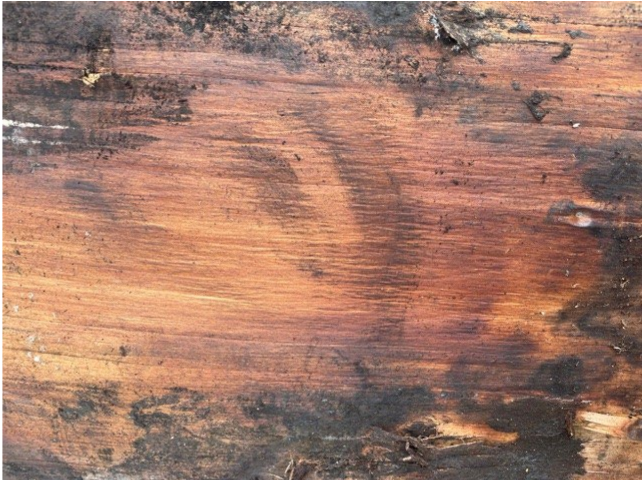
Figure 14 Example of Scorched Wood
