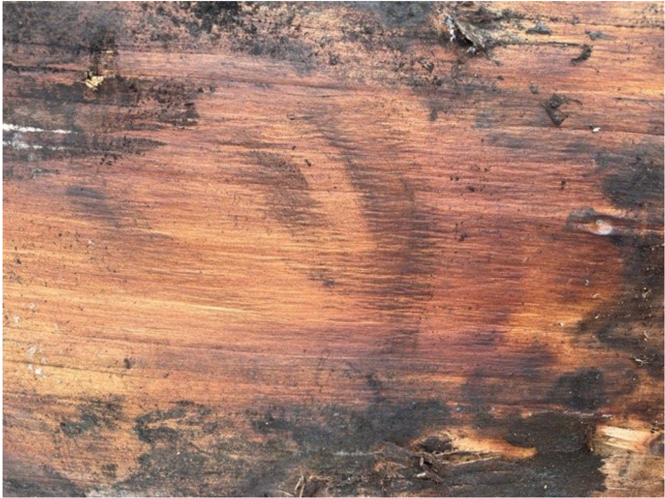
Figure 14 Example of Scorched Wood
