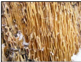
Tangential view of advanced honeycomb decay caused by O. tomentosa (Photo credit R. Reich).
