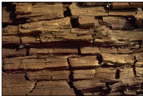
Longitudinal section of brown cubical decay.
