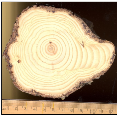
Cross section of Elytroderma infected trunk (Photo credit R. Reich).
