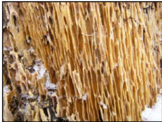
Tangential view of advanced honeycomb decay caused by
