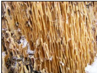
Tangential view of advanced honeycomb decay caused by O. tomentosa (Photo credit R. Reich).
