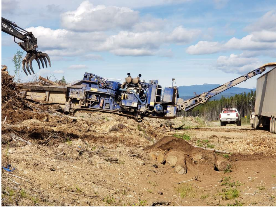
Figure 4. Peterson 5710 horizontal grinder.
