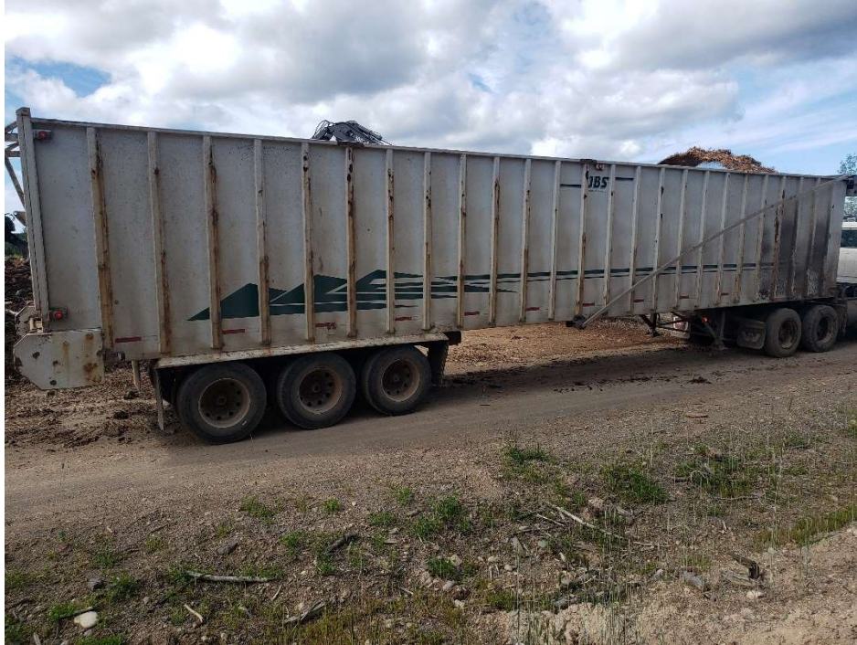
Figure 7. Tandem drive with truck with 53ft chain drive trailer.
