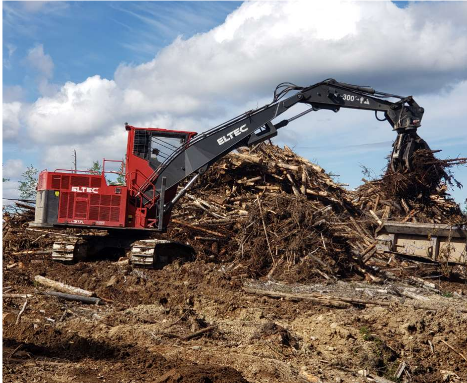
Figure 6. Eltec LL317 log loader.
