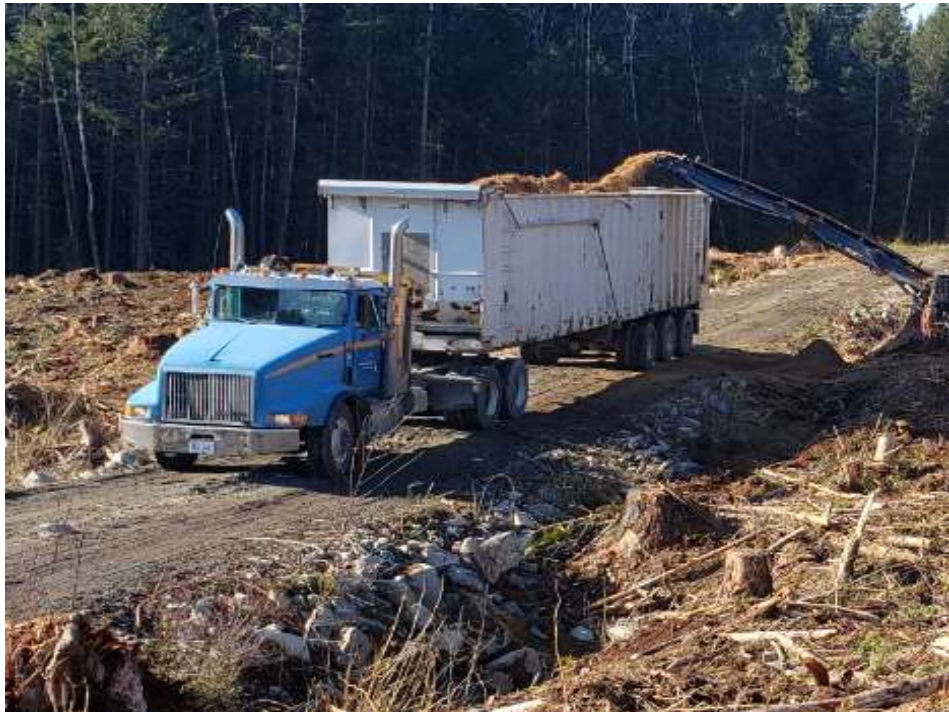
Figure 8. Tandem drive truck with 48ft chain drive trailer.
