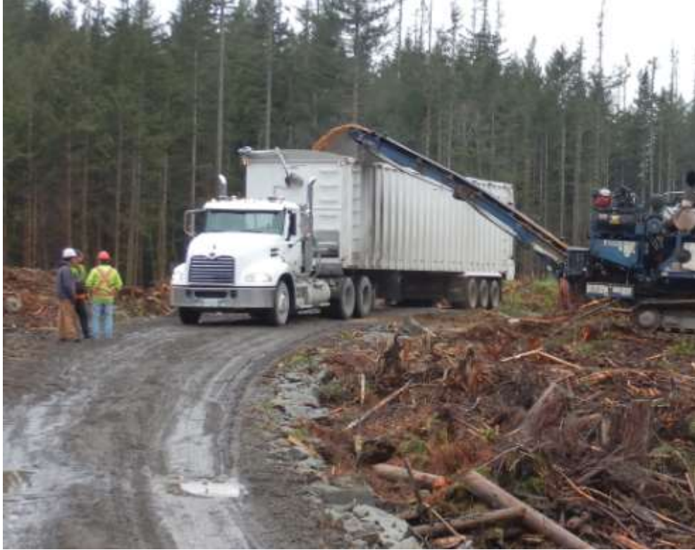
Figure 7. Tandem drive truck with 52ft chain drive trailer.
