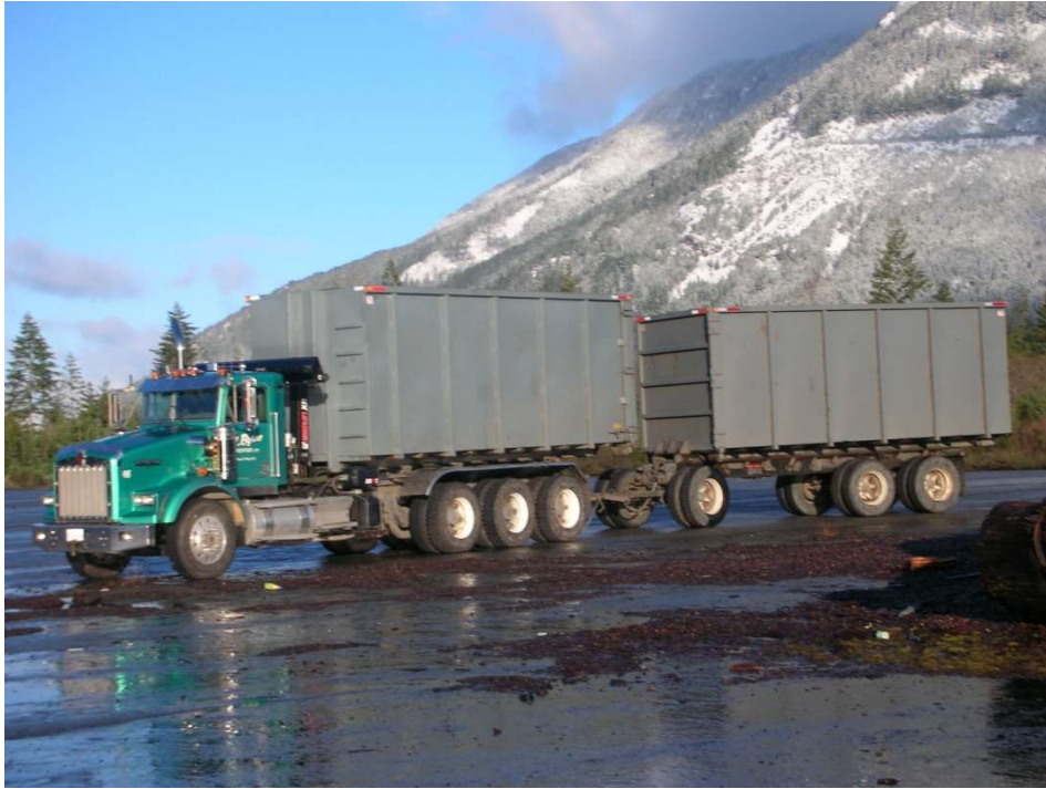
Figure 6. Tri-drive truck with dual bins.
