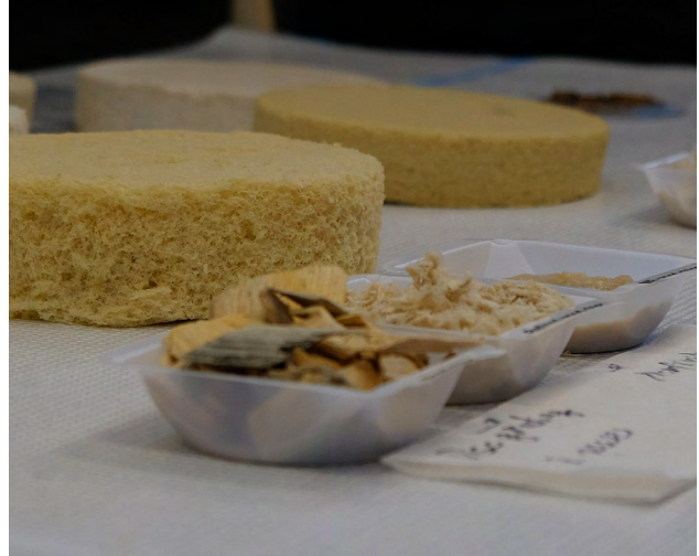
Above: Wood chips transformed into cellulose foams that can be used in insulation
