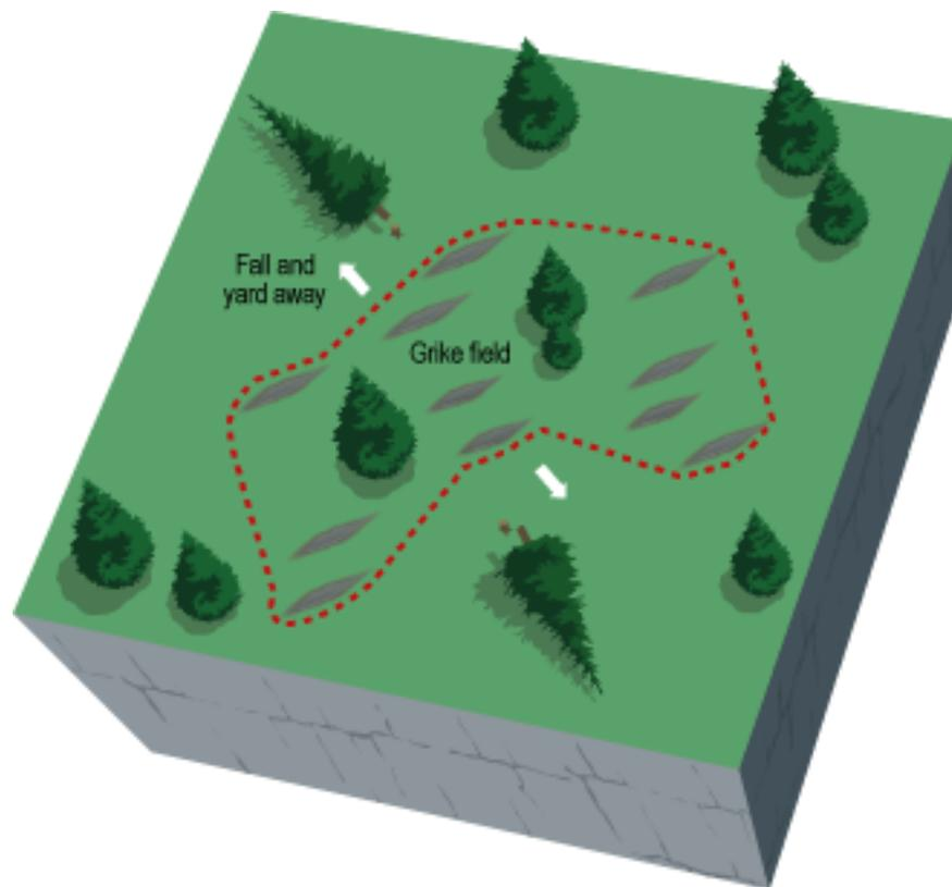
**Figure 11.** Example of treating a cluster of minor surface karst features as a single unit.
