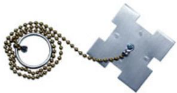
FIGURE 28. Relaskop angle gauge with basal area factor 3, 10, and 30.
