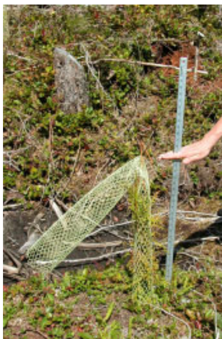
Figure 5. Vexar tube folded over at pin height by strong winds and heavy snow.
