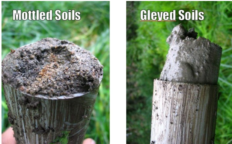
Figure 34. Examples of mineral soil with mottling or gleying effects.
