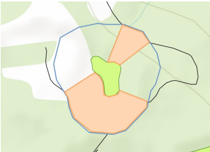
Figure 23. A 160 m segment of the wetland perimeter has a road within 100 m; 180 m of the wetland perimeter lacks roads within 100 m. Thus 47 % ( [160 / (160 + 180)] * 100 ) of the wetlands perimeter has road impingement within 100 m.
