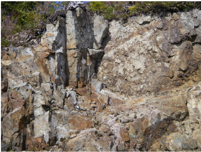
Figure 2. When rust staining is noticed in rock quarries or road prism culverts, managers need to determine whether the use of acid-generating rock is impacting water quality.
