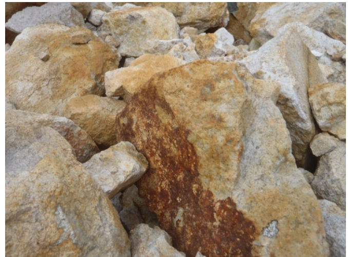
Figure 3. Typical iron staining in quarry rock. Fissures in acid-generating rock exhibit this rust staining on exposure to air and water. Where the rock is not fractured, staining may become apparent only after the rock is crushed.
