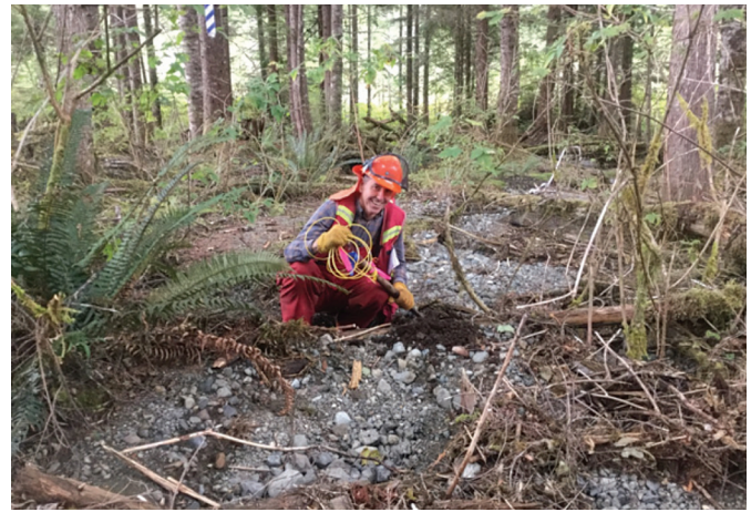
Figure 6. FREP assessor attempting to find an original S3 stream channel under sediments approximately 100 m downstream of a road crossing.
