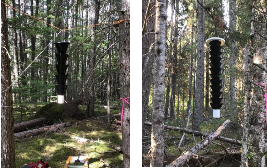
Figure 2. Multitrap, 5-unit (left); Lindgren funnel trap, 12-unit (right)
