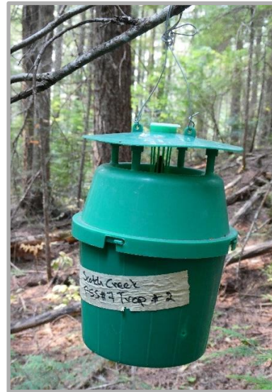
Milk carton trap for Douglas-fir tussock moth monitoring (left) and uni-trap for western hemlock looper monitoring (right).
