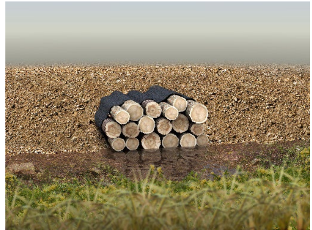
Photo #2: Use of three log and separation layer to maintain void to ensure water to pass freely.
