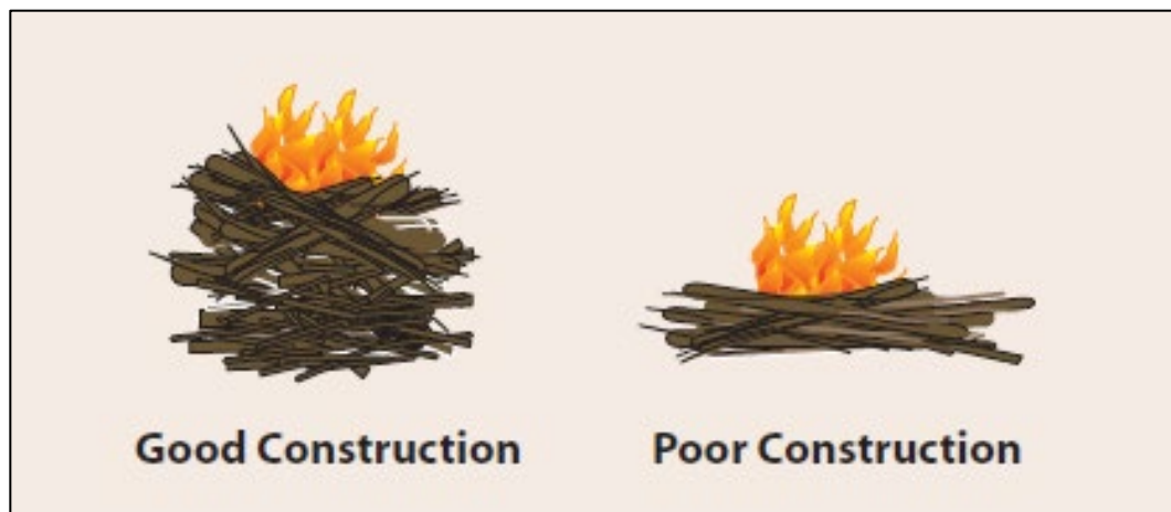
Figure 1. An example of good and poor pile construction. The good construction pile is stacked vertically with fine fuels at the bottom, covered with larger logs, for ease of ignition and optimal heat transfer. The poor construction pile is horizontal and has mixed fuel sizes at the base of the pile, leading to poor heat transfer.
