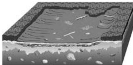
Compacted areas are areas on which there is evidence of compaction at the survey point and on 100% of a portion that is both greater than 100 m<sup>2</sup> in area and greater than 5 m wide.
