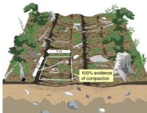
Repeated machine traffic must be counted as soil disturbance where there is 100% evidence of compaction in a 1m X 2m area on all sites, except those with low compaction hazard. Where the compaction hazard has not been assessed, repeated machine traffic must be counted as soil disturbance.
