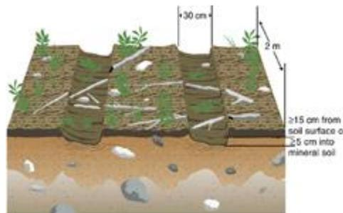
Wheel or track ruts 5cm deep X 30cm wide X 2m long are counted as soil disturbance on sites with high or very high soil compaction hazard or where compaction hazard has not been assessed.
