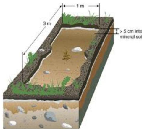
*Long gouges* are excavations into mineral soil that are a) deeper than 5 cm at the survey point and b) deeper than 5 cm or to bedrock on 100% of an area 1 x 3 m.
