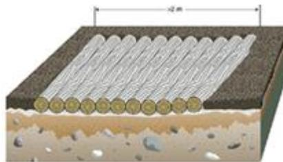
*Corduoyed trails* are constructed using logs and woody debris placed side by side to form a surface greater than 2 m in length and capable of supporting equipment traffic.
