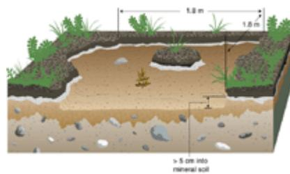
*Wide gouges* are excavations into mineral soil that are a) deeper than 5 cm at the survey point and b) deeper than 5 cm or to bedrock, on at least 80% of an area 1.8 x 1.8 m.
