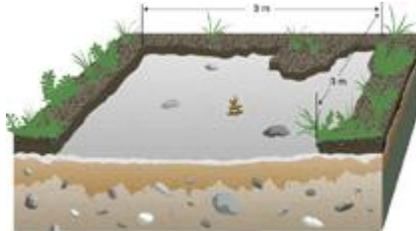
*Very wide scalps* are areas where the forest floor has been removed at the survey point and from over 80% of an area 3 x 3 m.
