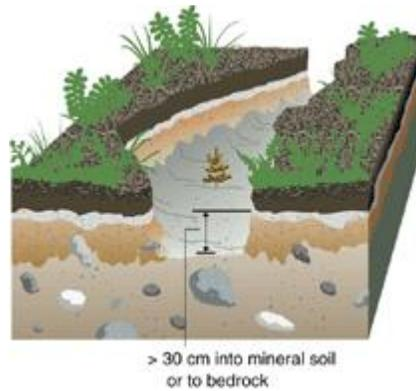
*Deep gouges* are excavations into mineral soil that are deeper than 30 cm or to bedrock at the survey point.
