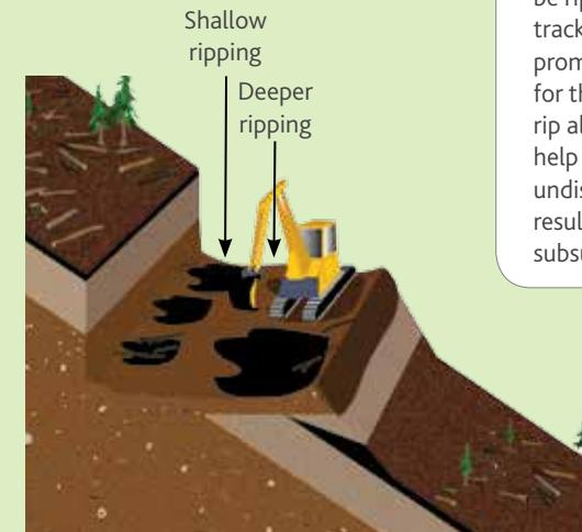
**2** The mid track position should be ripped deeper than the inner track (upslope) position. This will promote an outloping profile for the loosened soil. The shallow rip along the inner track will also help to prevent ripping into the undisturbed subsoil which could result in intercepting any functioning subsurface drainage.
