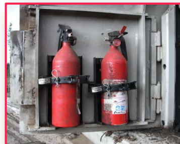
FIGURE 13. Fire extinguishers mounted on an excavator.
