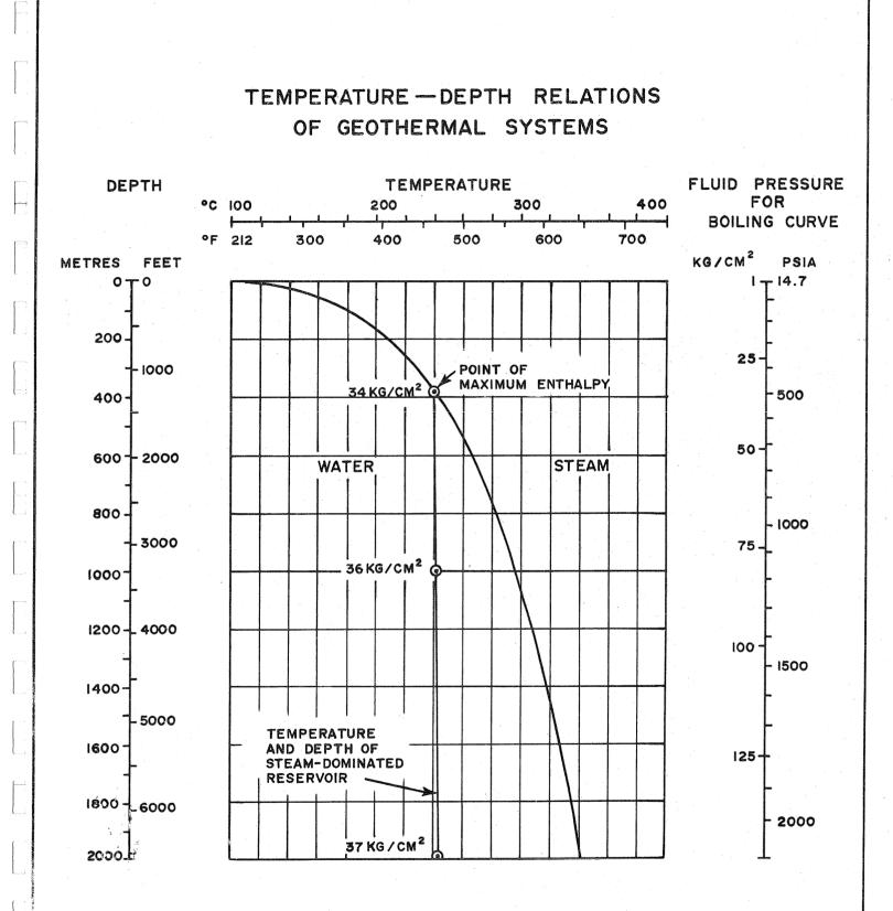
Adapted from (1) California Division of Oil and Gas (2) White, Muttler, Truesdell. In general a lithostatic pressure component derived from a seal is needed to lift the column of hot water up the well bore, where the delivery pressure is reduced mechanically and a portion of the fluid boils, or "flashes" to steam.
