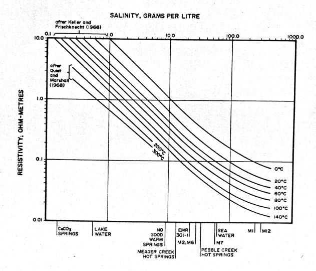
The effect of temperature and salinity on the resistivity of water. The salinities of cold sea water and lake water are plotted, along with samples of cold, warm and hot spring and drill hole waters from the Meager Creek Geothermal Area, B.C.
