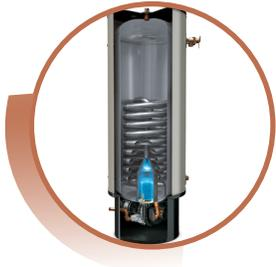
**What products are you regulating?** Storage-type water heaters with a rated storage capacity of 76 to 380 litres and an input of 75 000 Btu/h or less, for use with natural gas or propane.
