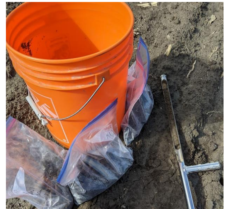
Figure 3. Soil sampling equipment; clean bucket, soil probe, ziplock bags, and permanent marker.
