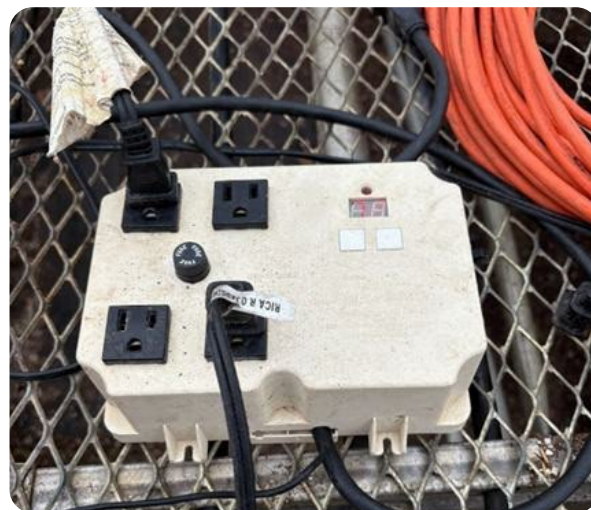
Figure 3. These professional grade heat mats are controlled by an external thermostat.
