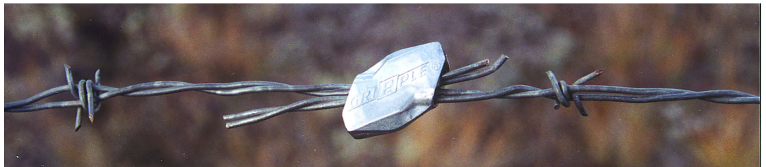
Figure 4 Knots and Mechanical Splice for Barbed Wire
