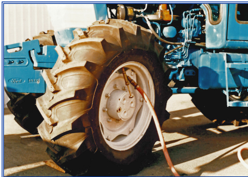
Water-calcium mixtures are pumped into the tire with the valve stem in the highest position.
