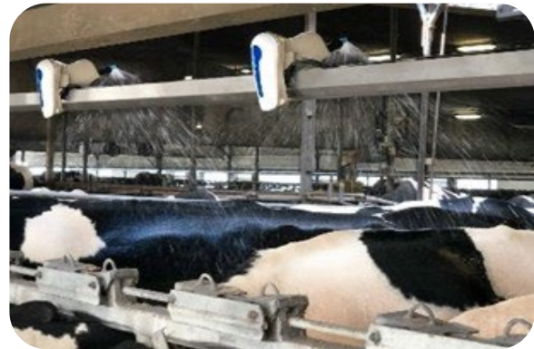
Figure 6. Soakers can sense whether a cow is within range (Agpro® Smart Soaker)
