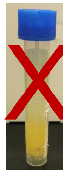
Virus transport medium with 'yellow color' indicating bacterial growth. DO NOT use if fluid is yellow
