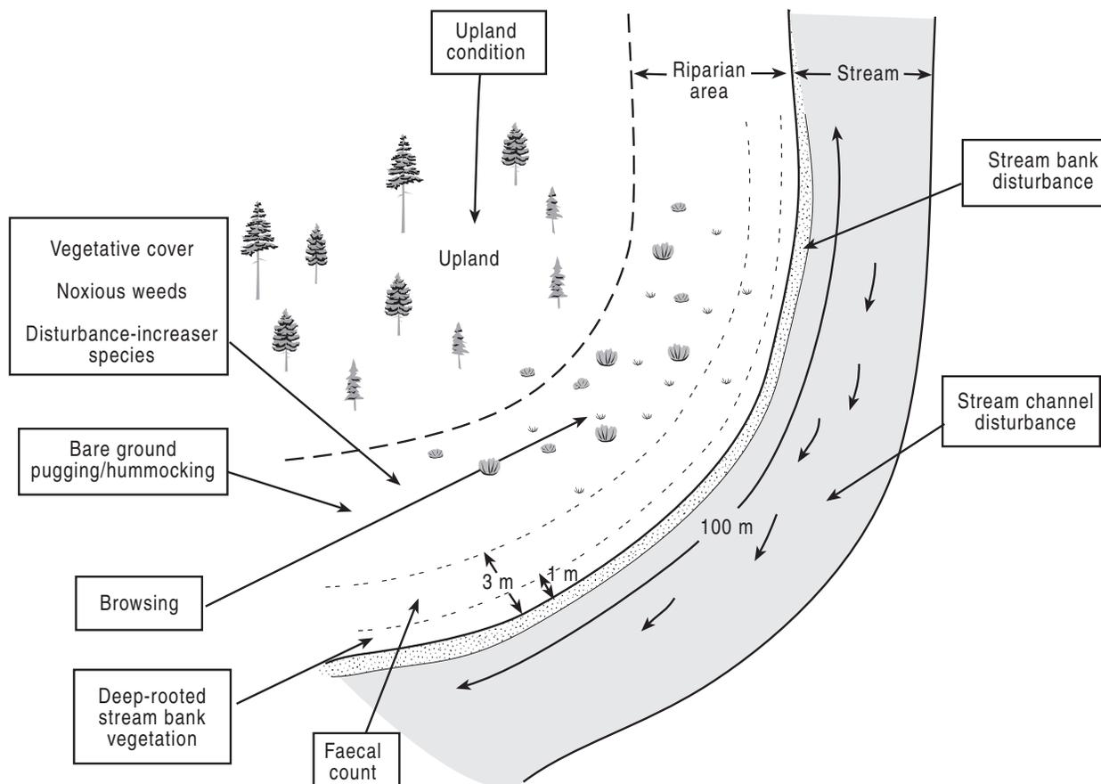
**Diagram 1.** Sketch showing the location in the stream channel or riparian area where the indicators were measured. Indicator values are averaged over a 100-metre reach.
