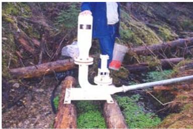
Ram pumps date back to the 1790's and early 1800's and utilizes the water hammer effect. It creates a pressure rise (water hammer) in a falling column of water by alternately opening and closing the column to free flow. Each time the water flow is shut off (quickly) the resulting pressure rise is used to pump a small volume of water. To operate, a Ram Pump requires:
