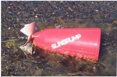
These pumps use the energy in flowing water (i.e., flow that's a result of gravity) to lift water above the supply. One example is the *Sling Pump* that rotates as the flowing water passes through the drive blades. It can deliver a volume and lift of water well suited for many livestock requirements. It is portable so multiple sites are possible with minimum setup. To operate, the pump requires:
