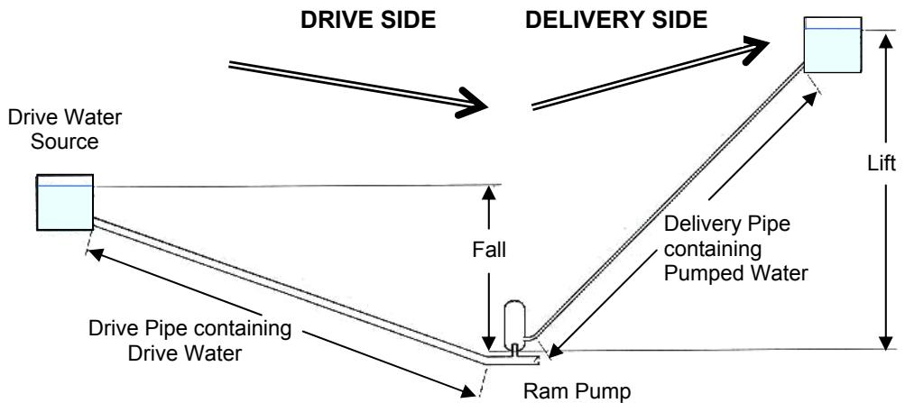
**Figure 9      Hydraulic Ram Pump**
