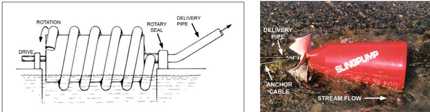
**Figure 5      Coil (Sling) Pump**
