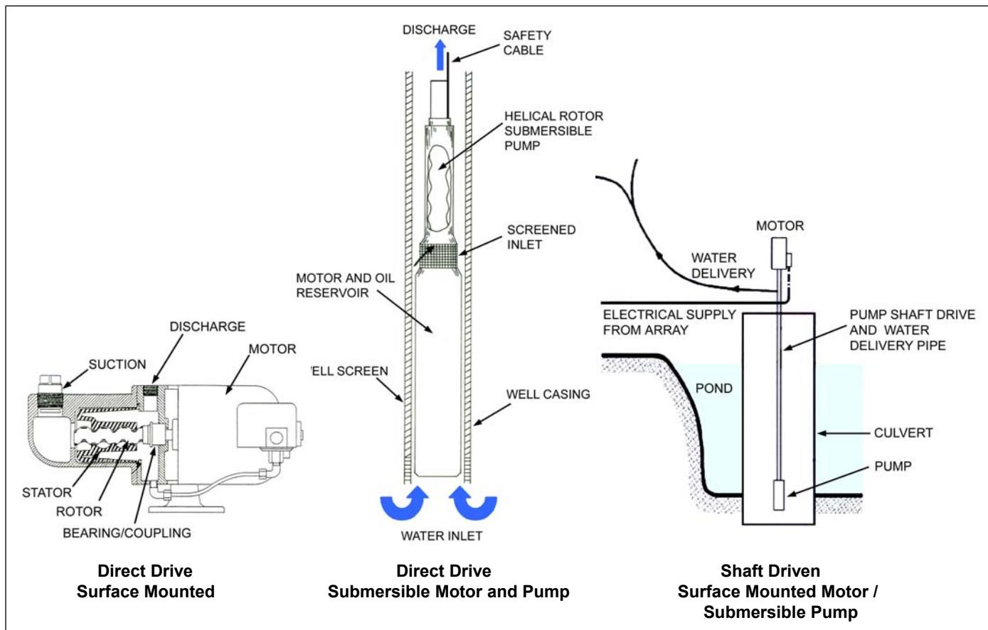
Figure 4 Progressive Cavity Pump Drive Options
