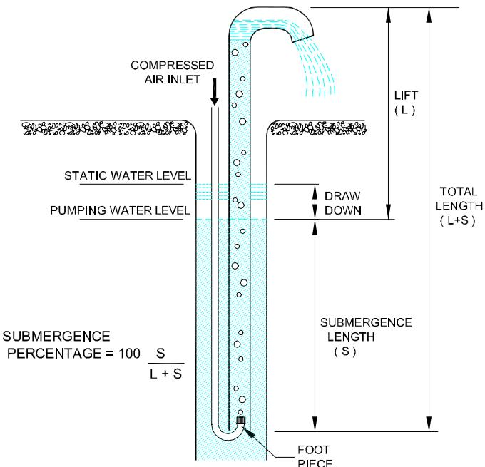
**Figure 8      Air Lift Pump**
