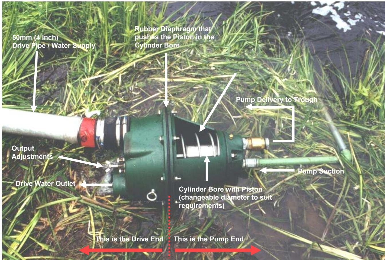
**Figure 10      Modified Hydraulic Ram Pump (*Glockemann 320*)**
