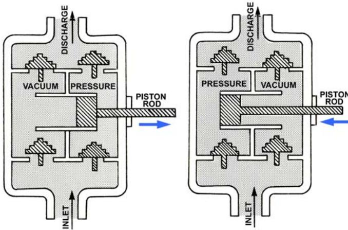
**Figure 2 Double-Acting Piston Pump**
