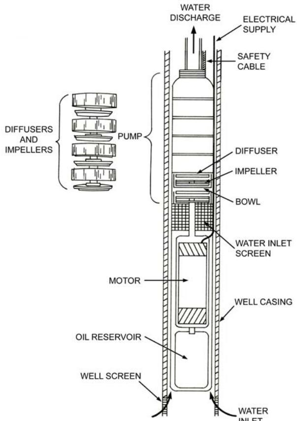
Submersible Turbine-Centrifugal Pump
