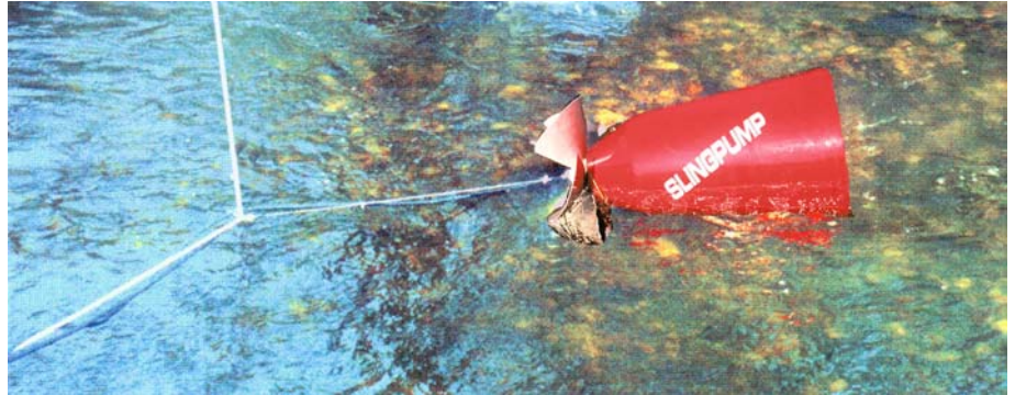
Stream-Powered Pump ( Sling Pump )
