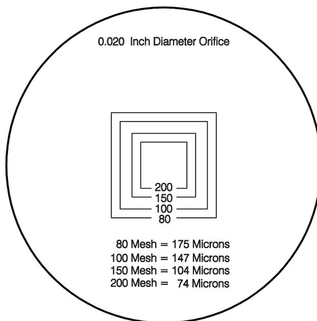
Figure 10.2 Comparison of Screen Mesh Sizes with a 0.20" Emitter Orifice
