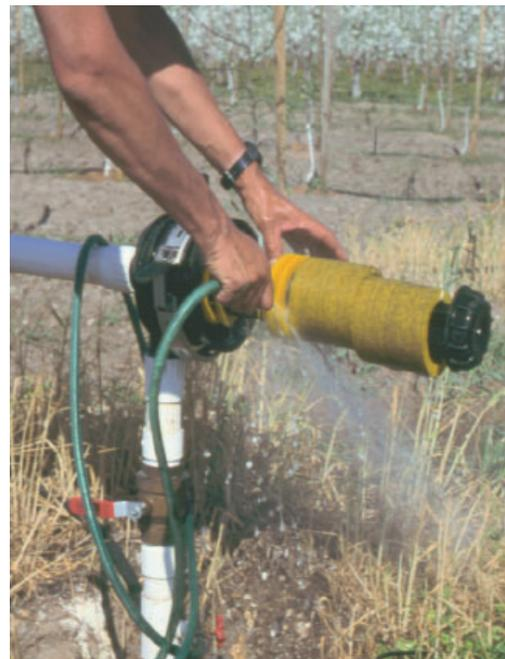
Manual Cleaning of a Disk Filter
