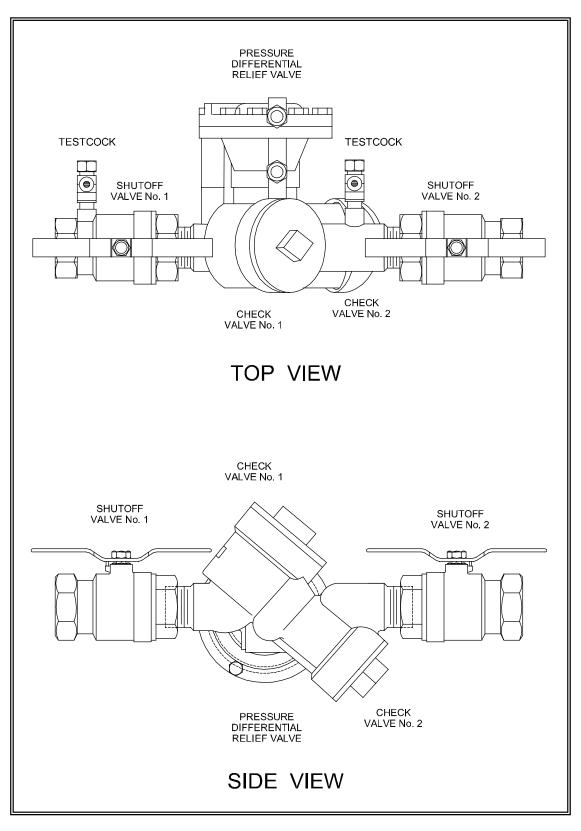
Figure 4.2 Reduced Pressure Backflow Prevention Principle Device
