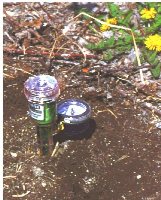
Figure 1 Tensiometer in the soil after installation
