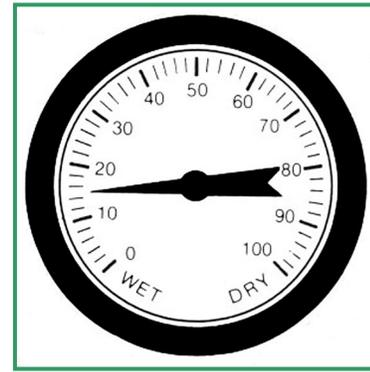
Figure 2 Tensiometer Gauge
