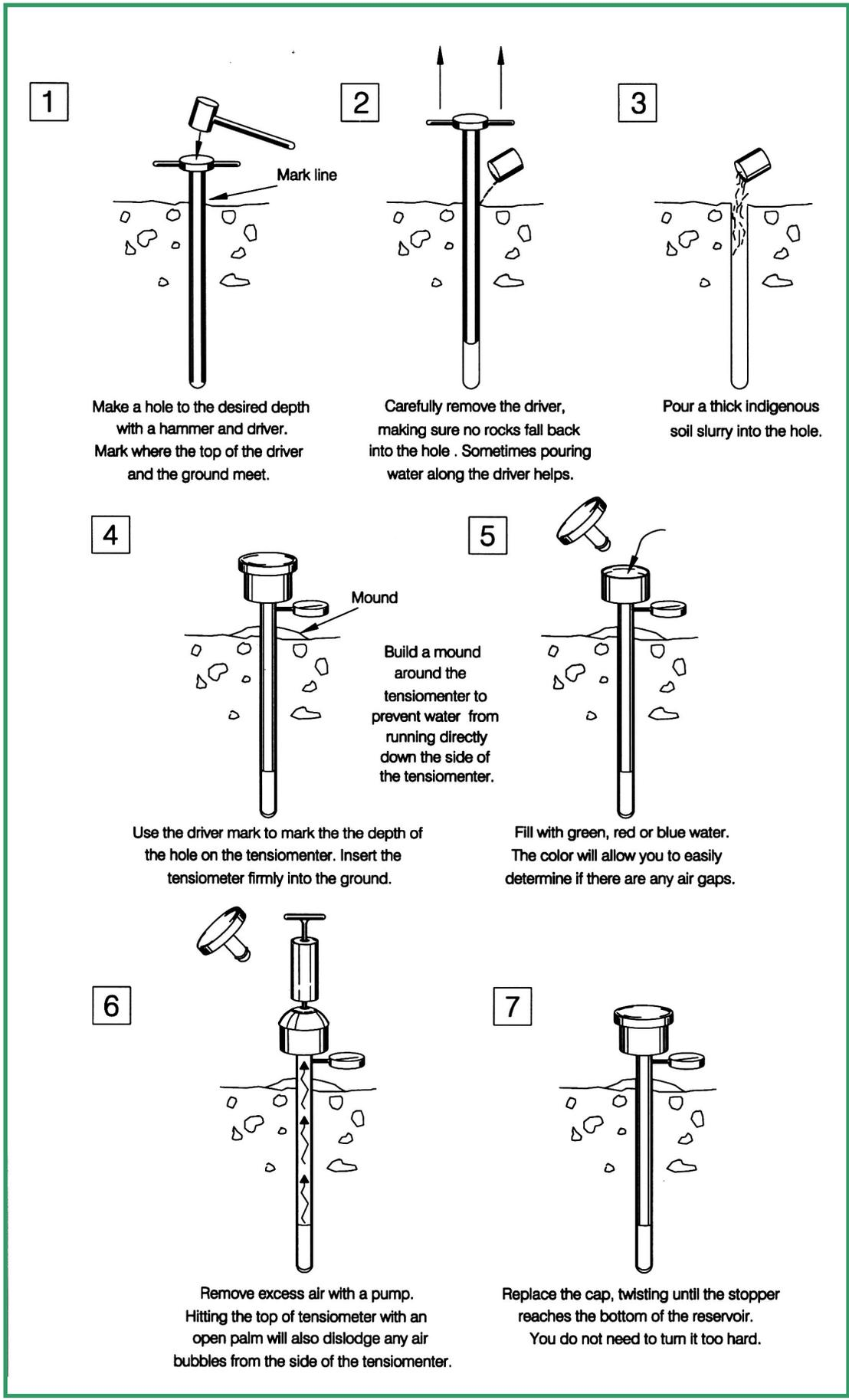
Figure 4 Tensiometer Installation Procedures
