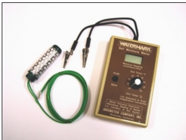
Figure 4 Electrical Resistance Block
