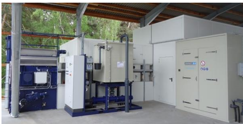
Photo of the DGM conveyor belt dryer and water wash drying digestate in Germany.
