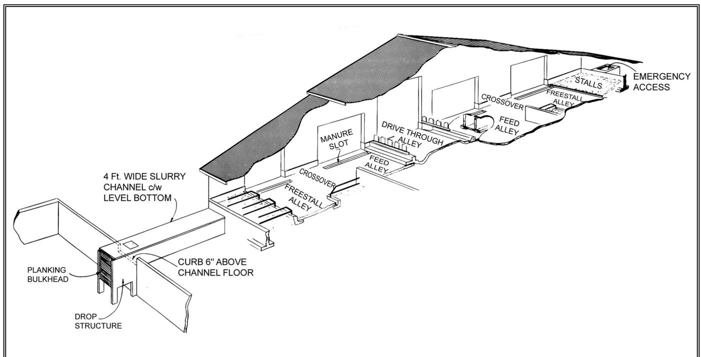
Gravity flow slurry channels are popular as a method of dairy manure transfer in liquid manure handling systems. Proper management of slurry channels is essential to their satisfactory operation. With good design and careful management, trouble-free operation is easy to realize.
