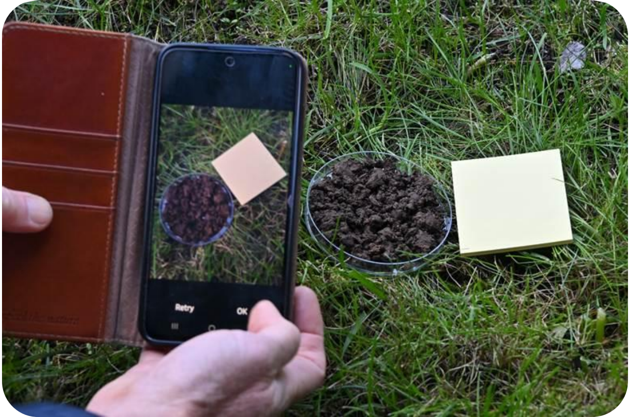
Figure 4. Soil and reference material photographed for determining soil colour using the LandPKS smartphone app
