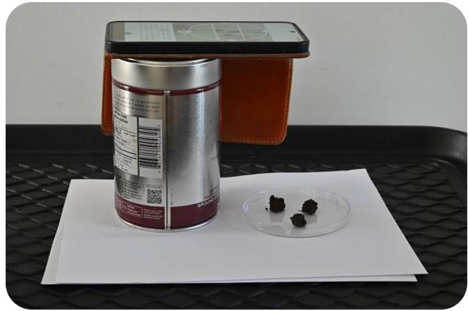
Figure 9. Setup for aggregate stability testing using the SLAKES smartphone app.
