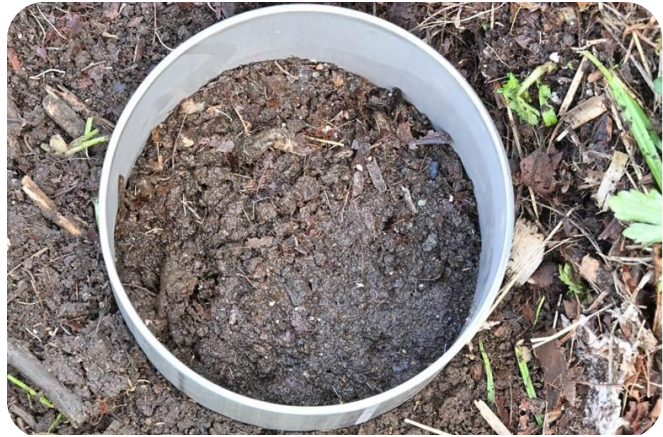
Figure 3. The infiltration ring when the infiltration test is completed and the soil surface is glistening.
