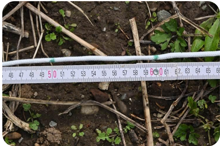
Figure 2. Soil cover being measured using the line-transect method.
