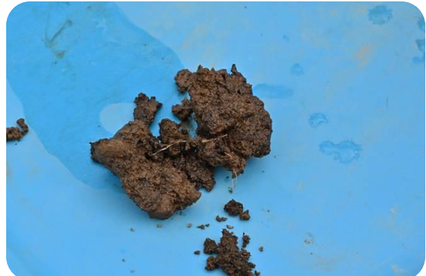
Figure 4. A saturated soil aggregate broken apart to determine the level of saturation.
