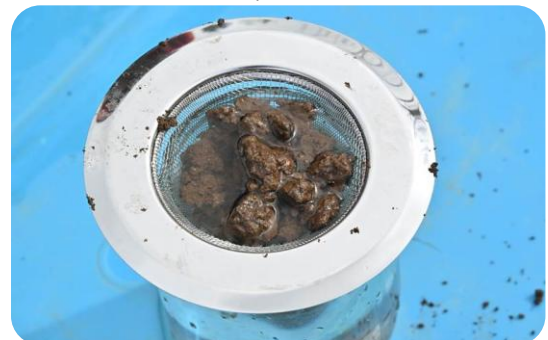
Figure 6. Soil aggregates submerged in water to determine aggregate stability using the strainer method.
