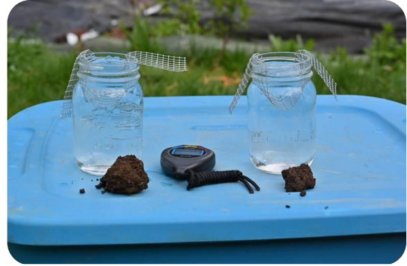
Figure 1. Soil aggregates prior to being measured for aggregate stability using the jar and wire method.
