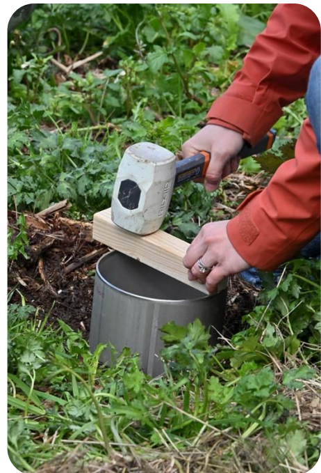
Figure 1. An infiltration ring being inserted into the soil.
