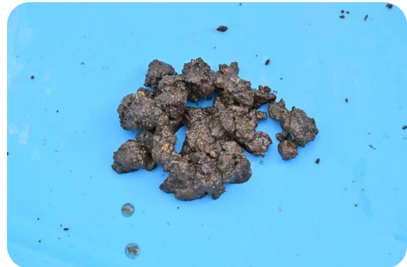
Figure 8. Saturated soil aggregates after being removed from the strainer to determine the level of aggregation.
