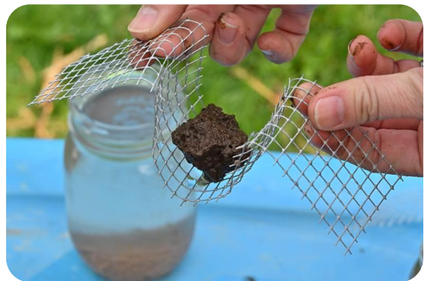
Figure 3. A saturated soil aggregate after being removed from the jar.
