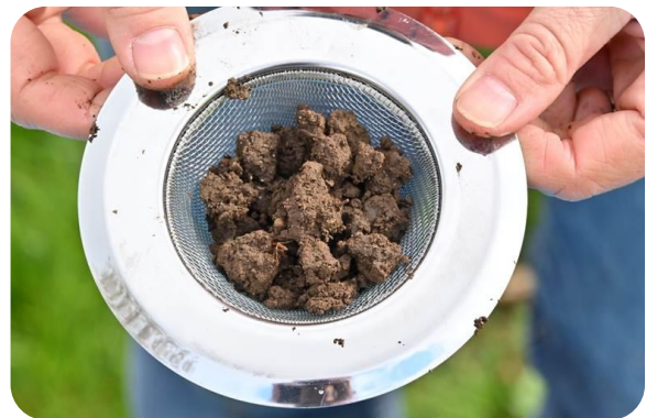
Figure 5. Soil aggregates prior to being measured for aggregate stability using the strainer method.
