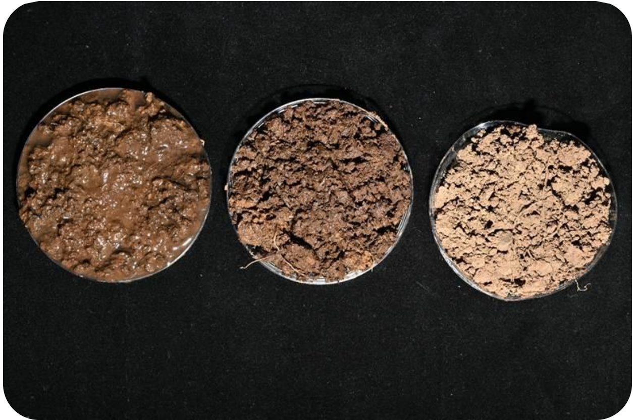
Figure 1. A handful of soil at three different moistures for the purposes of determining soil colour: dry, moist, and wet
