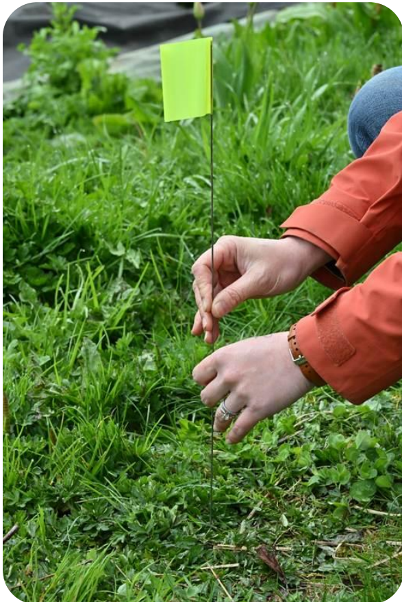
Figure 1. A wire flag being inserted into the soil to determine penetration resistance.
