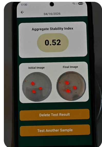
Figure 12. The aggregate stability index score using the SLAKES smartphone app.
