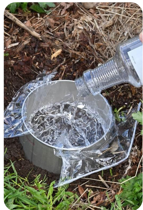
Figure 2. Water being poured into an infiltration ring lined with plastic wrap.
