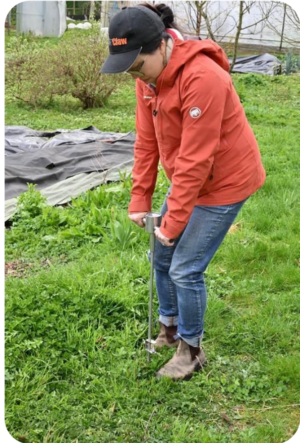
Figure 2. A penetrometer being inserted into the soil to determine penetration resistance.
