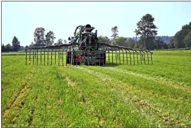
Figure 3 Trailing hose manure application
