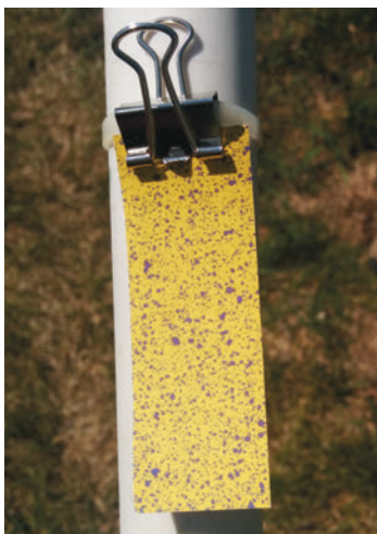
Figure 15: Spray card to evaluate pesticide drift
