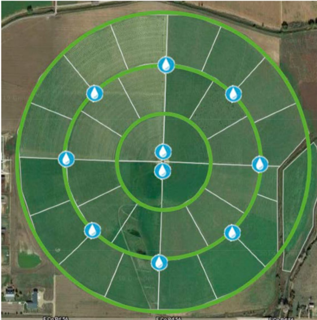
Figure 6. MiG system design on a 200-acre pivot including high-tensile concentric fences (green), moveable polywire paddock fencing (white), and watering locations at Colorado State University. Polywire locations represent areas associated with the given water points and are often further subdivided into 2 or 3 smaller paddocks depending on animal numbers and current forage supply (Figure by Casey Shawver, retrieved from PastureMap mobile application).
