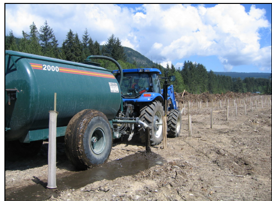
Photograph 22: Tractor towed liquid tanker being used to fertilize a row of poplar trees
