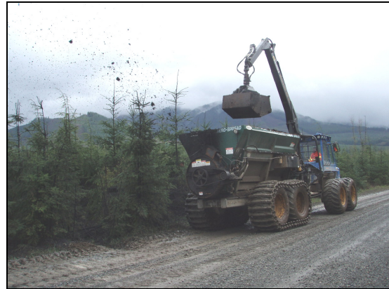
Photograph 31: Aero-spread box mounted on a Rottne forwarder for forestry applications
