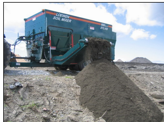
Photograph 3: Tub mixer used to combine feedstocks to achieve a BGM
