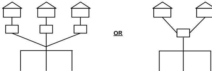
**Separate Sewerage Systems (Not a Combination of Systems)**
